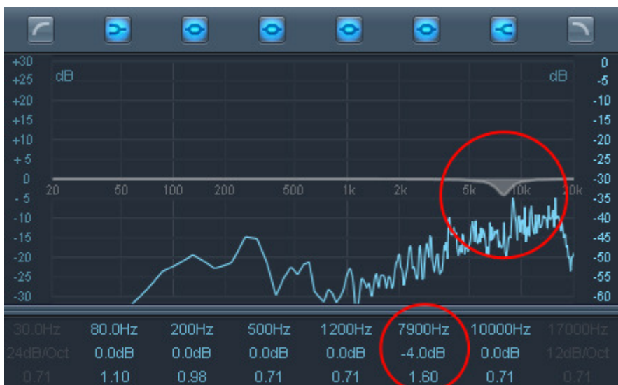
2. Light cut with 4 dB at 7900Hz, this hihat sounds a lot smoother now!
